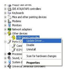
3. Select "Install the software automatically (Recommended) and follow the prompt screens. If installing the driver automatically doesn't work, go back to your Device Manager and do another right click on USB-Serial and select Update Driver but this time select "Install from a list or specific locations (Advanced)" make sure it said "C\SpecWare, if not click, Browse, and point to the location where SpecWare is saved and follow the prompt screens.
